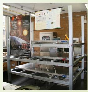
When a charged particle passes through a telescope chamber, the electronics of the device are activated to determine the crossing time. This is accounted by the time during which the signal is kept above a fixed threshold level
